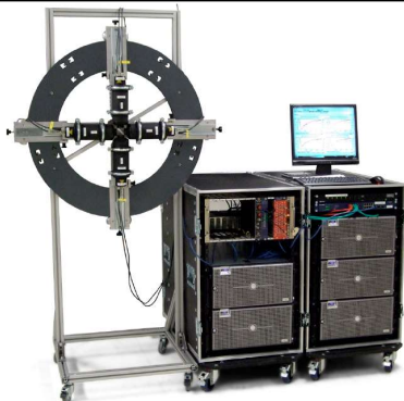
FIG. 4. (Color online) A photo of the current setup. In the two mobile racks are the four recording computers and the server as well as network, high voltage, and control devices. On the left side the four detectors arranged around a sample are visible.
